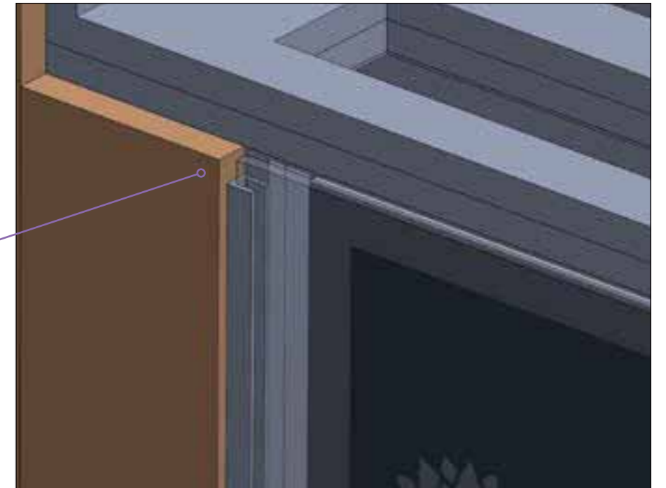
Lexan slides into steel C sections. Can be removed by opening top cupboard
